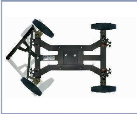
with single ended, corrected steering geometry allowing a minimum circular movement of 258 cm / 9' 4" inside diameter.
